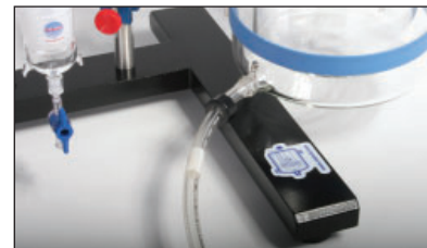
Connecting to Reservoir's inlet
