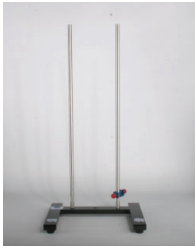
Assembling Steel Base, Support Rods, and attaching a Universal Stand Clamp (SSteel)
