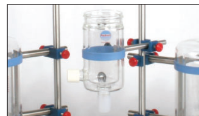
Attaching assembled Heart Chamber to a Support Rod
