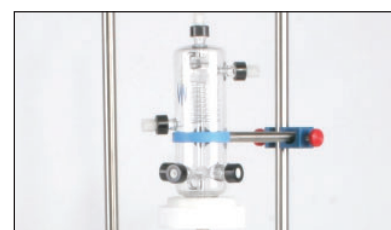
Attaching assembled Direct Perfusion Core to Support Rod
