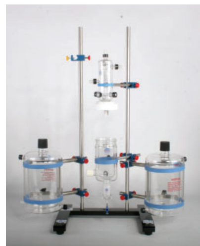
Attaching the Universal Stand Clamp (Nylon) for the 2-Way TNV "Y" Manifold
