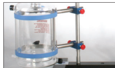
Attaching the other assembled Water Jacketed Reservoir on the left Support Rod
