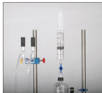
Connecting Damping Syringe to the Direct Perfusion Core
