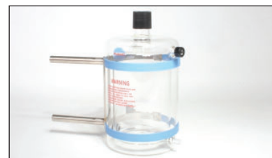
Orientating and securing Double Ring Clamp
