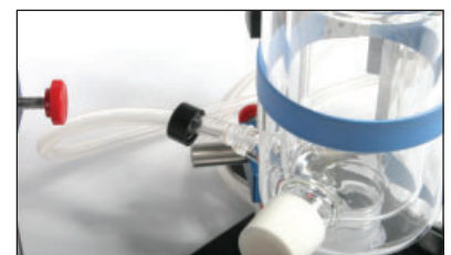
Connecting to Heart Chamber's inlet
