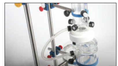
Connecting Heart Chamber to Perfusion Core
