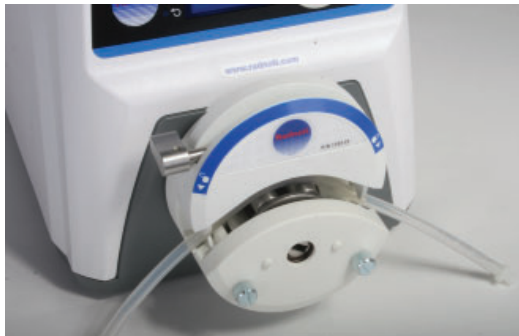
Moving lever left to load Pump Tubing
