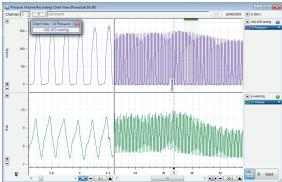
*Above*: Loop View (right) generated from pressure and volume data in Chart View (left) provides online and offline analysis of all or selected PV Loops with ESPVR and EDPVR values.
