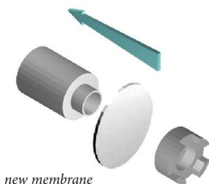
3. Place new membrane over top of tip and press onto cover cylinder. Trim excess membrane.
