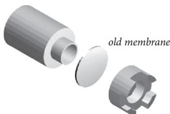
2. Remove old membrane and clean cylinder and tip.
