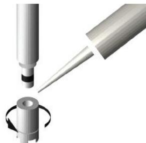
4. Use syringe (supplied with electrode) to place a small amount of R001069 Electrolyte filling solution into the lower part of the electrode then screw back onto the main body. Excess filling solution will be extruded.
