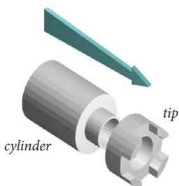
1. Unscrew the lower part of the electrode then pull to remove tip from cylinder.
